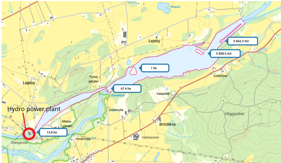
Figure 25: Reservoir size of Karsefors hydro power station (Lanmäteriet, 2023)
